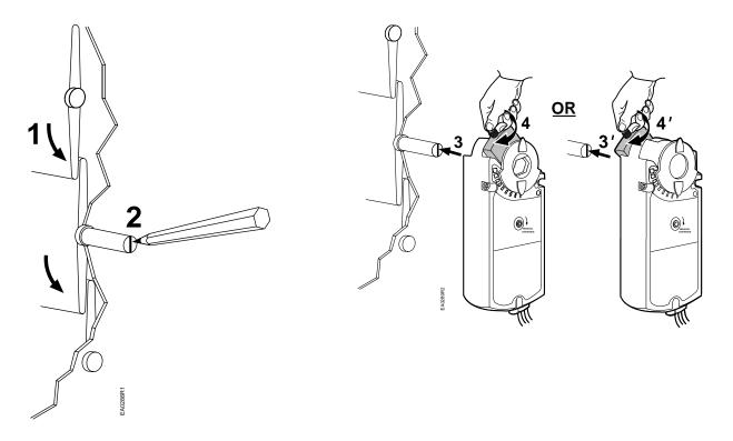
Place the actuator on the shaft with the damper blades in the desired 0 position. Tighten the middle screw so that the shaft is in the center of the shaft adapter opening.
